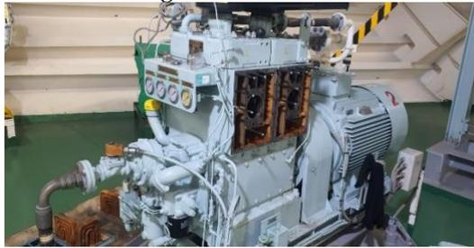
Gambar 6 Proses overhaul main air compressor
