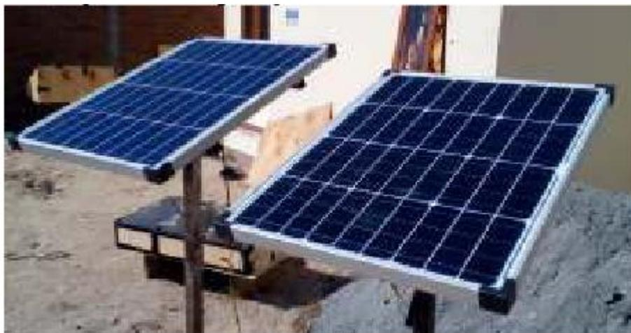
Gambar 1.1 Set up panel surya polycrystalline dan monocrystalline
